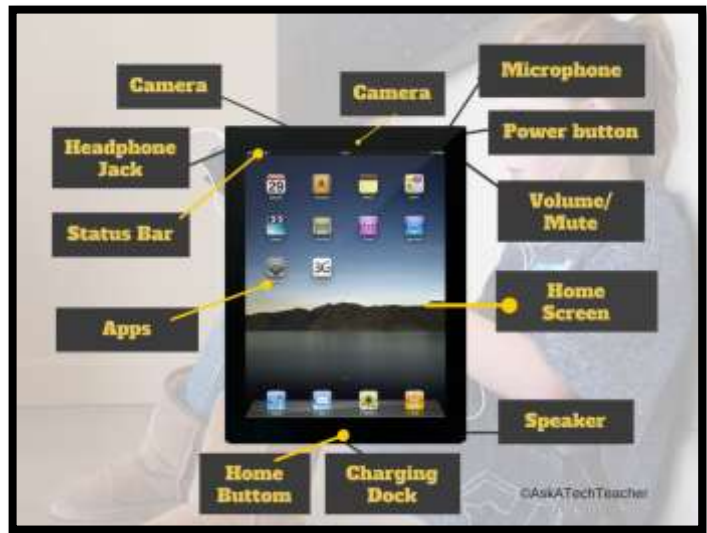
Figure 14a—Parts of computer; 14b—Parts of iPad
